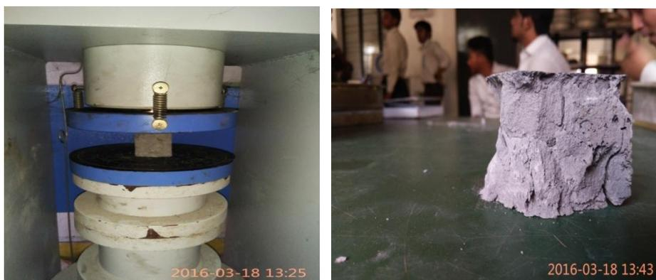
**Figure-1:** Specimen under compressive testing set up and Fracture surface of typical geopolymer material.
