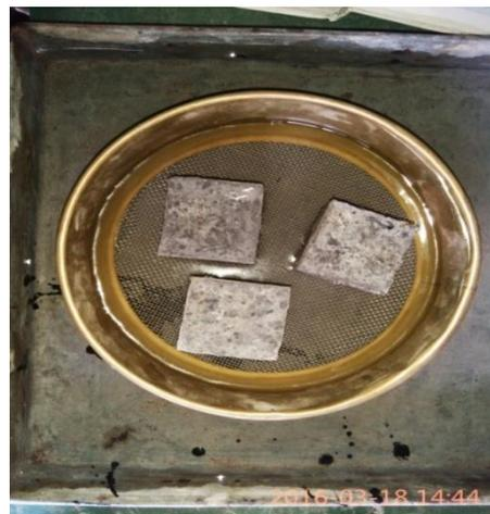
**Figure-3:** Specimen subjected to unidirectional sorption
