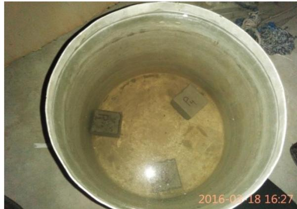
**Figure- 2:**Specimen submersion in fresh water
